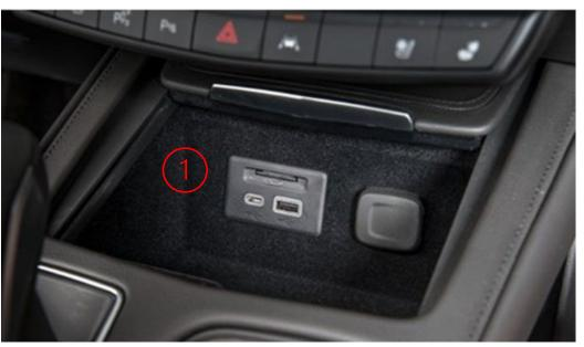
With the vehicle powered off, you can eject the existing SD Card from the slot by giving a gentle push on the SD Card and then pulling it out.
